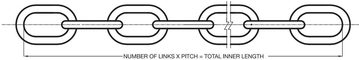
**AMH** kiln chains are supplied in materials ranging from carbon steel to high temperature stainless steel. The welding process is done robotically and supplied in cut-to-size lengths.
