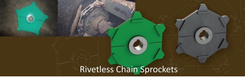
ANH rivetless chain sprockets can be manufactured either to standard design or with a machined relief area which keeps the chain from riding out of the pocket, preventing premature wear. Our sprockets and tail idlers are manufactured by combining a standard abrasion resistant 400 BHN plate and mild steel hub.
