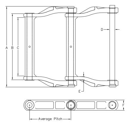
HD480 Cast Drag Chain AMH HD480 chains come in Cast Alloy 8630 QT380-400 material. Our chain is assembled using machined 4140 through-hardened pins with riveted construction. This chain features a cast integral sidebar making this link one piece fully cast. Chain comes with center point pre-greased barrel and 1" rivet.
