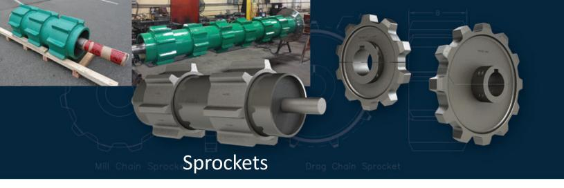
ANH sprockets are made from AR400 BHN plate. They can be supplied in several different sizes and hub configurations. Our in-house drafting department will design sprockets specific to your requirement. We offer the shortest lead time in the industry. We are able to do this with our wide range of AR400 plate inventory, in house burning table, CNC mill and lathe.
